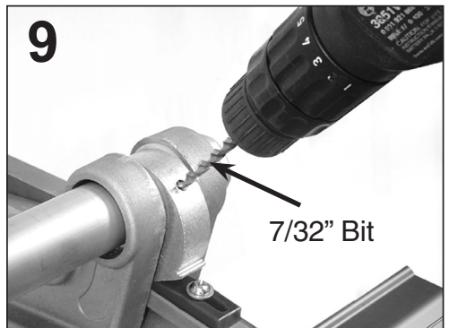
9 Drill new hole into cam tube. Use hole in cam for a pilot hole. Reinsert screw.
